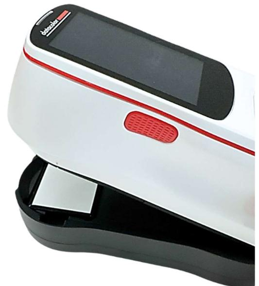
7. Press 'Calibrate' to measure the White Tile. *(see page 27 for calibration screens)*
