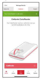
5. Place the Swipe Colour Match Tool against the flat surface you want to measure and tap the button on the device or on the screen to get your results.
